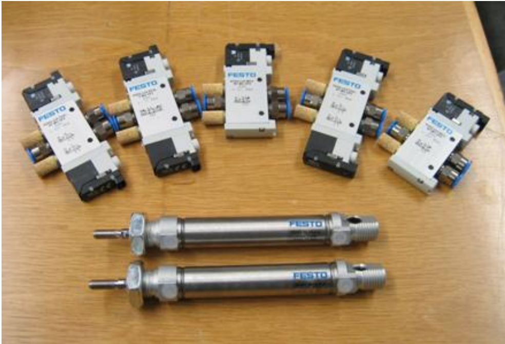
Figure 3: Pneumatic valves and suspension absorbers from one of our sponsors FESTO
