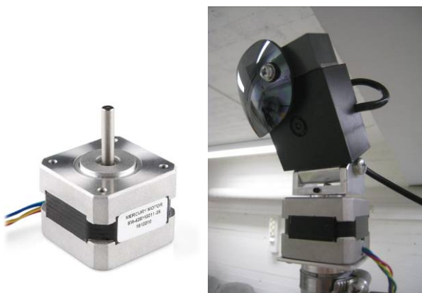
Figure 4: On the left: the stepper motor. On the right: the camera head with re-encapsulated Logitech 5000 with a sun glass.
