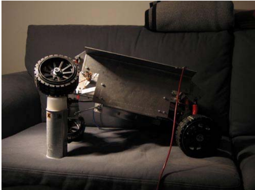
Figure 2 Torsional twist system allows robot to climb over large obstacles. It balances tilting of the chassis to keep machine vision sight on the field.
