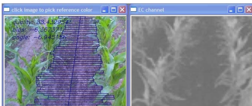
Figure 8 Row Detector B debug output is printed over original image. Right is shown the EC channel from which the ground is detected.
