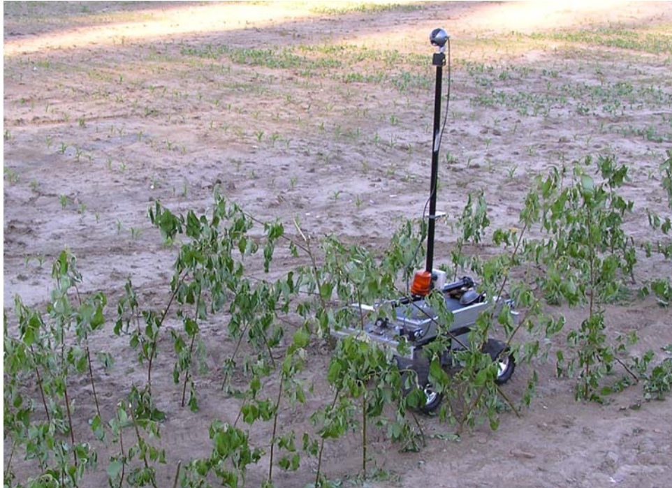
Figure 1-1: Test field in Finland built from birch branches
